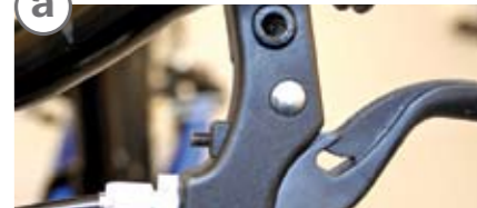
Brake cable barrel adjuster (below) and reach adjustment screw (above)
