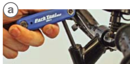
Tightening the stem height bolt
