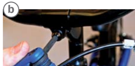
Tightening handlebar clamp bolt
