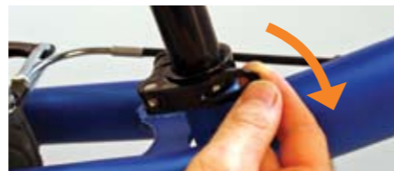
Open Quick-release lever. ONLY if required – loosen / tighten tension adjusting nut
