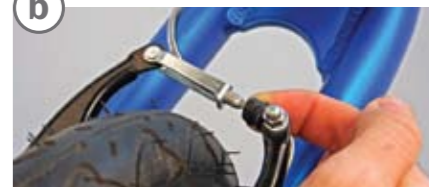
Sliding the dust cover away from lead pipe
